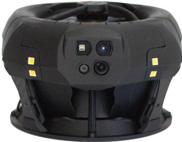
*The Dronut X1 from Cleo Robotics is the first professional-grade, bi-rotor ducted-fan drone – a drone without exposed rotor blades.*
