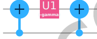
Fig. 36. An IBM Quantum Experience score illustrating an implementation of the MaxCut edge gate (71).
